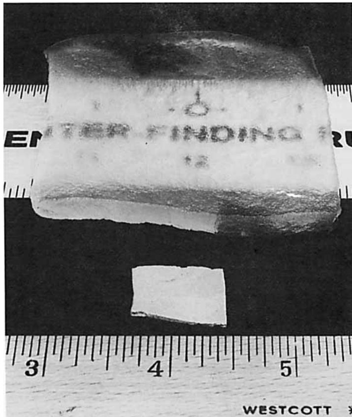
Fig. 2. Photograph of Super-Slurper enmeshed in PTFE composite membrane, showing a sample (bottom) that was dried at ambient room conditions and an equivalent sample (top) originally of the same dimensions that was swelled to equilibrium in excess water.
